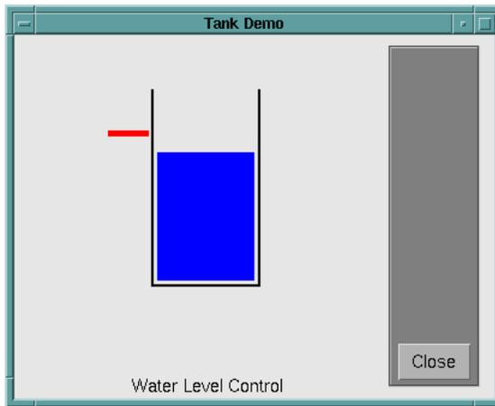
A controller for the water level in the tank needs to know the current water level and it needs to be able to set the valve. Your controller's input is the water level error (desired water level minus actual water level), and its output is the rate at which the valve is opening or closing. A first pass at writing a fuzzy controller for this system might be the following:
