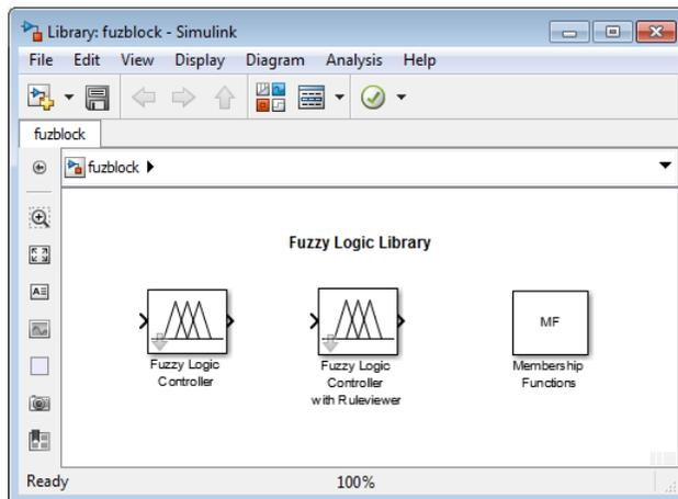
The Fuzzy Logic Toolbox library contains the Fuzzy Logic Controller and Fuzzy Logic Controller with Rule Viewer blocks. It also includes a Membership Functions sublibrary that contains Simulink blocks for the built-in membership functions.
