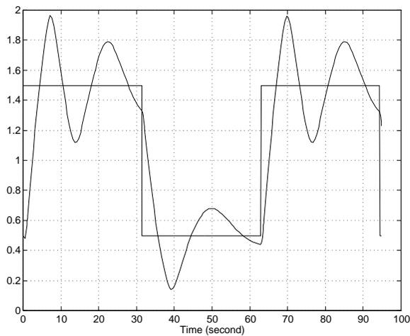
You need to add another input, the water level's rate of change, to slow down the valve movement when it gets close to the right level.
